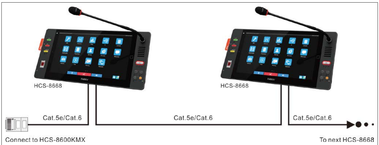
Figure 3.2.7 Daisy-chain connection between HCS-8638/8669/8668/8679 series Paperless Multimedia Congress Terminals
